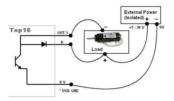
Each output is the collector of a transistor which effectively connects the output to 0V (when output is ON) and will sink up to 250mA (all outputs on) or 350mA (single output on). When the output is OFF it is a high impedance.
