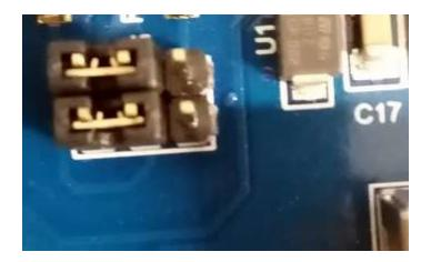
Programming mode. The Jumper Links connect UPDI to the Serial TX and RX.
